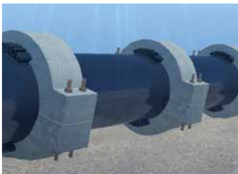
Fixing a sinker or thrust block to the pipe.
