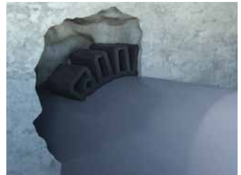
Anchoring the pipe to a concrete wall such as a manhole or tank.
